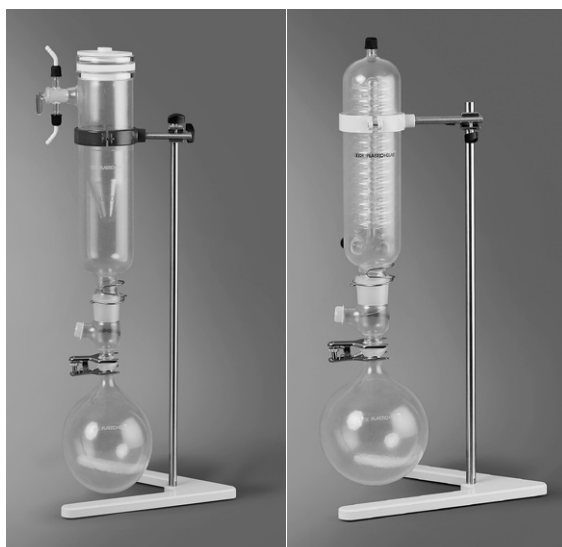
Fig. 4.16: Type C (left) and type S (right) condenser assemblies
