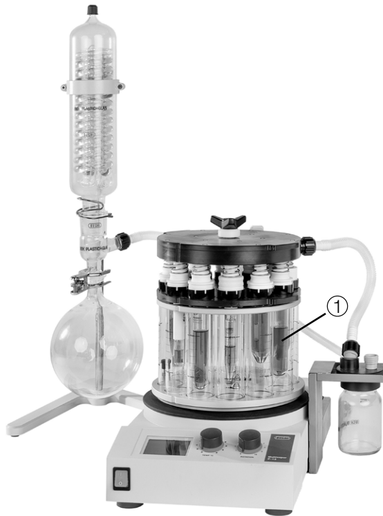
Fig. 4.8: Multivapor with the crystal rack
