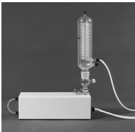
Fig. 4.20: Cooled receiver with type S condenser
