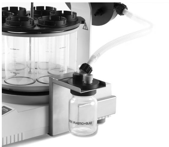
Fig. 4.17: Woulff bottle installed
